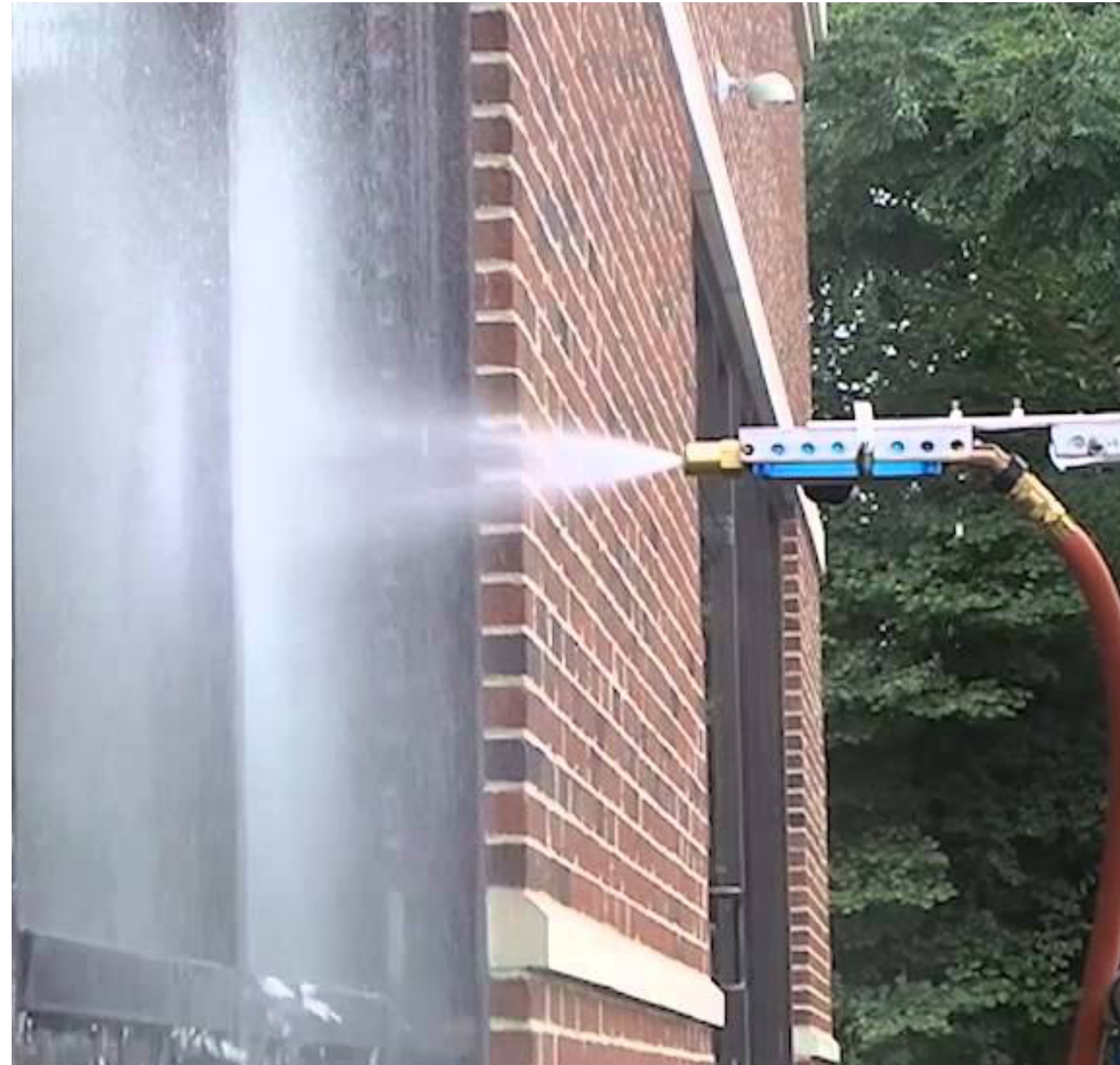
Testing a Window for Leaks
